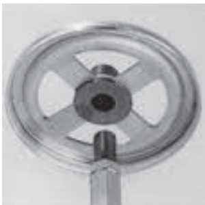
Shaft guide bearing made with a self-lubricating closed bush in molybdenum bisulphide polyamide and stainless steel shaft with ceramic insert at the point of wear.
